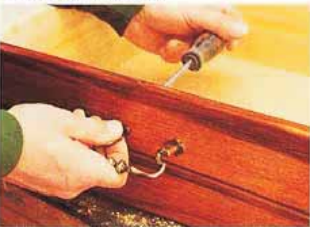
29 Fit the drop handles from inside the drawer.
