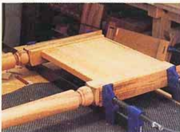
18 A couple of sash cramps will hold the joint closed while the glue sets.
