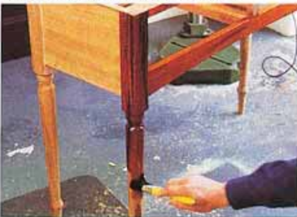
26 Brush on a coat of spirit stain then wipe off the excess with a cloth.
