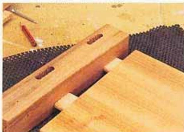
17 Put glue into the mortices rather than on the Beadlock strip.
