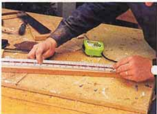
19 Use a flexible steel rule to set out the front rail curve.
