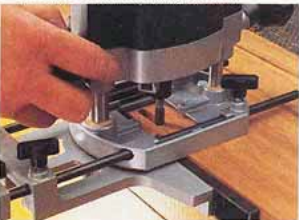
24 Cut slots in the top of all the rails to take the fixing buttons.
