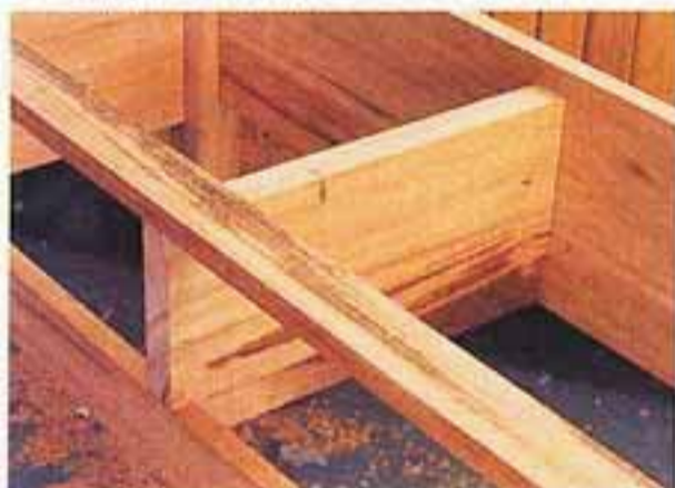
16 Cut and fit the central drawer divider. I used conventional dowels to fix it.
