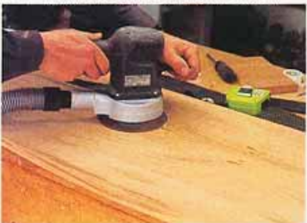
22 Sand the top to remove the machining marks and give a smooth, fine finish.
