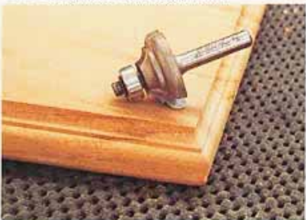
23 Use router cutters in combination to form the top edge profile.
