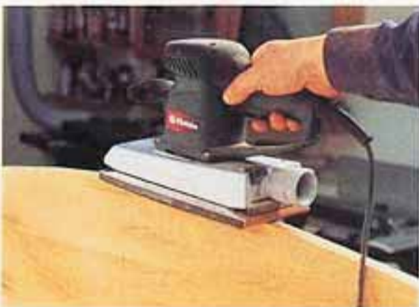
21 Use the orbital sander to clean up the convex edge of the top.
