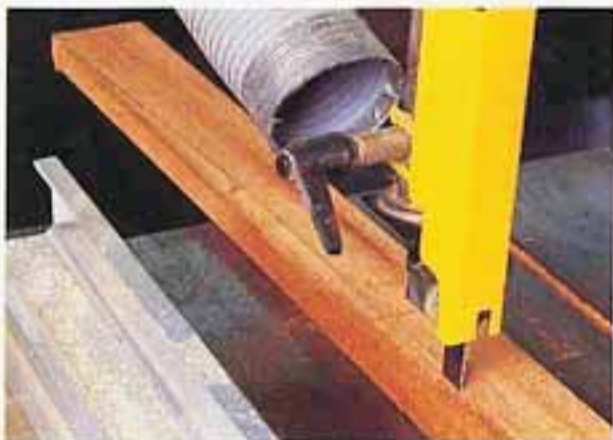
20 When you've got the shape right, cut the curve carefully on the bandsaw.
