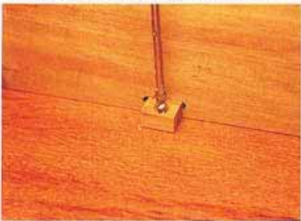
28 To fix the top down, screw the buttons into place in the slots cut previously.
