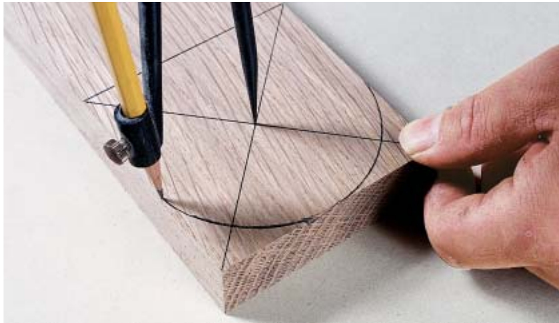
Photo B: Mark the outside circle before drilling the pivot hole.
