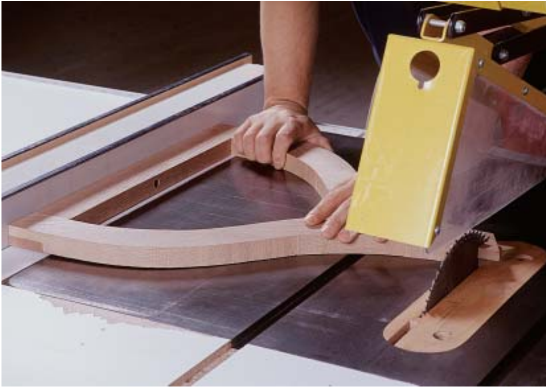
Photo H: After you've glued the cross bar to the harp and cut off the nibs, run the cross bar against the fence to cut the harp bottom. This ensures that the bottom is parallel to the cross bar.
