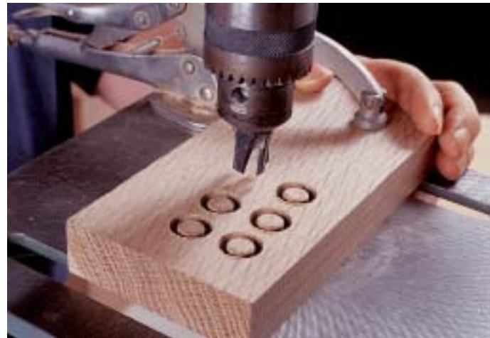
Photo D: If you cut your own plugs, you can match the grain direction and make the plugs almost invisible. Clamp the stock to the drill-press table so the workpiece doesn't spin.
