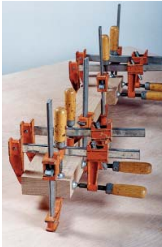
Photo A: Clamp across the joints to register the sides of the footpads with the sides of the feet.
