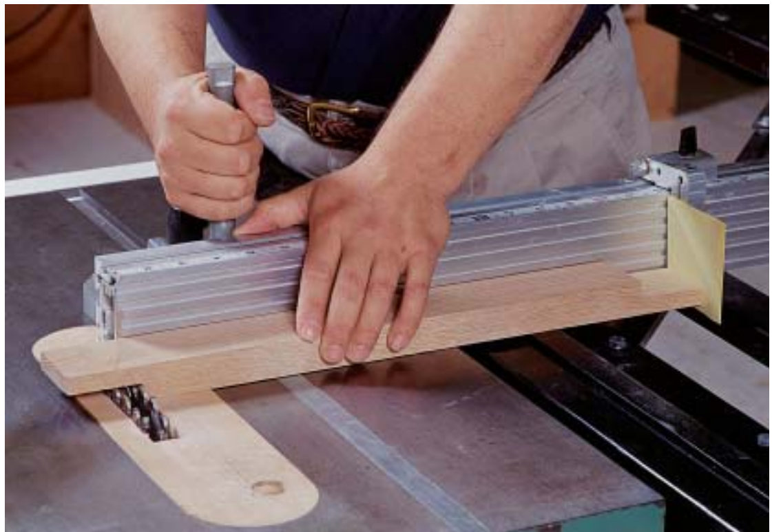
Photo F: Run the harp against the fence and cut the top shoulders square.
