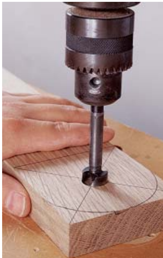
Photo C: Forstner bits leave clean entry holes even in difficult wood. Back up the exit hole with a piece of scrap so the exit is clean.
