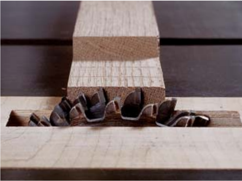
Photo E: Cut the joint slightly thick, then turn the practice piece over to see the difference between the blade and the remaining work.
