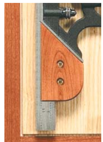
Combination square. A small angled block with a shallow kerf is all you need to capture a combination square.
