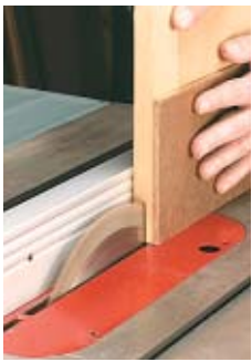
▲ This jig lets you cut the open mortises without having to adjust the fence. For details, go to page 8.
