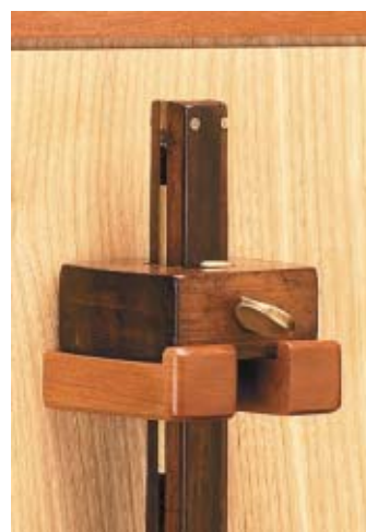
Marking gauge. For this marking gauge, a notched block supports the head, and a small lip keeps the tool from sliding off.
