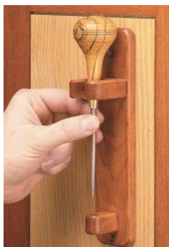
Scratch awl. An open hole traps the handle of this awl. And to protect your hands (and other tools), the point sits in a base.
