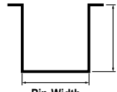
Pin Width 12.7mm (1/2") Pin Depth 20mm Max
