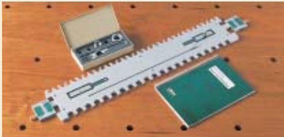
Ellipse and Wave joint patterns Maximum stock width: Ellipse: 23-1/4" Wave: 22-1/4"
