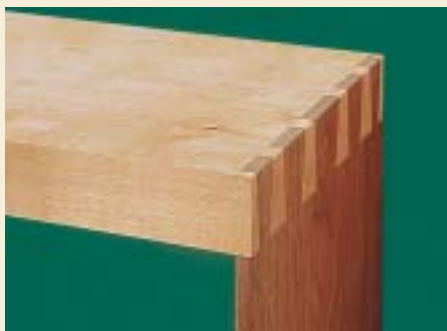
The Leigh Dovetail Jig can join pins and tails of different thickness up to 1-1/4".
