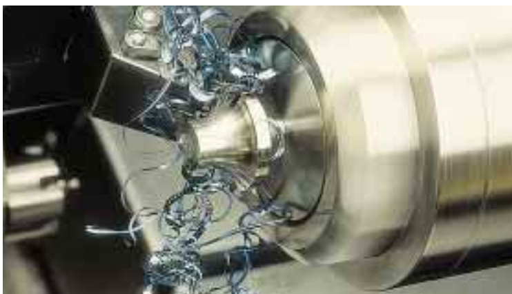
A bit is born - turning the body of a CMT Round Over Bit on a Swiss automatic lathe.
