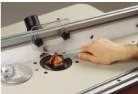
Using our bent wrench to change bits from the top of the table is quick and easy
